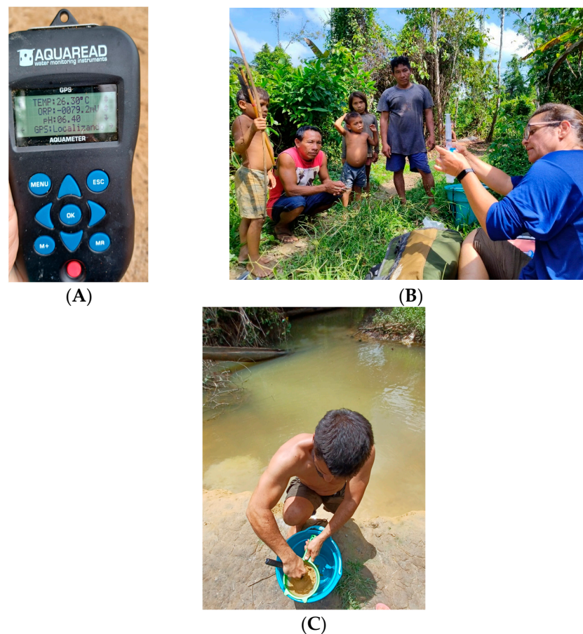
Figure 2. (A) Probe with some water measurements. (B) Water collection. (C) Stream sediment collection with sieving.
